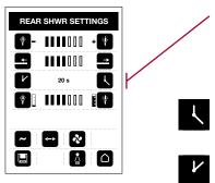
The shower duration for both the rear and lady shower can be modified individually. You can adjust the shower duration to between 15 and 25 seconds. The shower duration is adjusted in 5-second increments. The selected shower duration is displayed in the centre.
