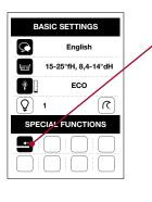
Press "Retract spray arm" to retract the spray arm again without the nozzle. You can clean the opening for the spray arm with a damp cloth.
