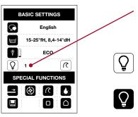
The white LED display provides lighting at night. Press "LED display" repeatedly to choose from 4 brightness settings or to deactivate the indicator.
