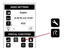
The thermal cleaning cycle on the shower toilet can be started manually without a reminder from the appliance.
