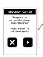
The remote control switches to the "Odour extraction" menu. Proceed as described in section 10.13, replacing the odour filter automatically.
