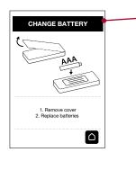
If only the instructions for replacing the battery appear on the remote control and the backlighting on the display is off, the batteries must be replaced immediately.
