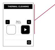
The remote control switches to the "Thermal cleaning" menu. Proceed as described in section 10.9, Thermal cleaning, automatic.
