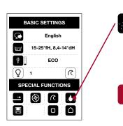
The decalcification program descales all parts that carry water. Press "Decalcification" to open the menu. Corresponding instructions on the remote control will guide you through the decalcification program.
