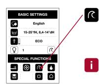
Thermal cleaning flushes the entire water-carrying system on your shower toilet with hot water to eliminate bacteria and germs.
