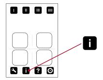
Demo mode allows you to perform a convenient demonstration or function check on the shower toilet without you having to sit on the appliance. Open the cover and place the splash guard in position.
