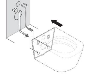
We suggest using the TOTO connecting set SP10695UN for hidden connections WASHLET™ RW, RX, SX GL 2.0, EK 2.0 to prepare the water connection on Geberit frames with empty conduit (located on the left hand side 50 mm from the center of the frame at the same height as the fixation bolts).
