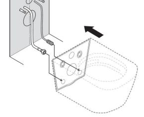
We suggest using the TOTO connecting set SP10695UR for installation frame for WASHLET GL 2.0 and WASHLET EK 2.0 with hidden connections to prepare the water connection on Geberit frames with empty conduit (located on the left hand side 50 mm from the center of the frame at the same height as the fixation bolts).
